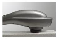
(bounce up and down). When this happens either slow the machine down or apply a moderate amount of pressure until the head stops pattering.
